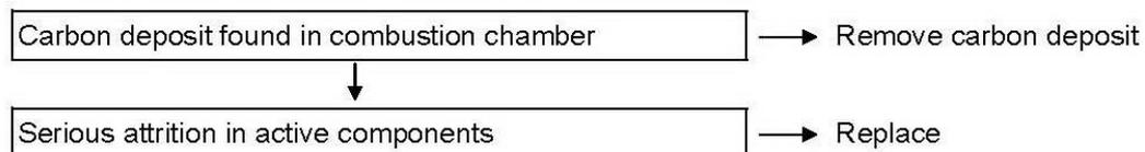
**Example 5: The machine is working normally, but the efficiency of cracking is very low**
